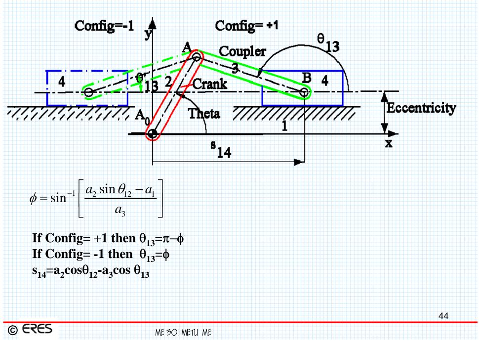
Example: Slider-Crank mechanism
