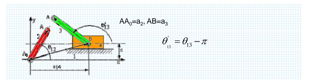
$A_0 A = A_0 B + B A$  loop closure equation (vector loop equation)
