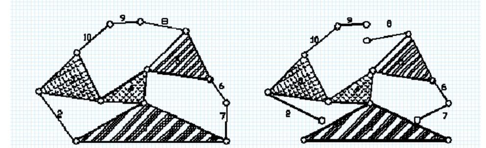
j = the number of joints in the open kinematic chain + the number of joints removed.
