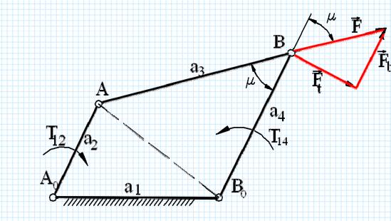
Transmission angle is a kinematic quantity which gives us an idea on how well the force is transmitted
