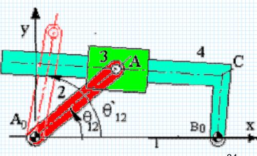
**Inverted Slider-Crank Mechanism**
